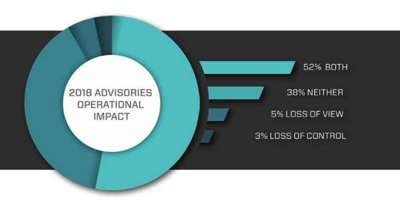
Vulnerabilities which lead to both a loss of view and control occur in the core of traditional control networks affecting both field devices (PLCs, RTUs, etc.) as well as management devices such as human-machine interface (HMI) systems and engineering workstation (EWS) software. This means that over half (60%) of ICS-related vulnerabilities can cause an operations outage, at least for the component affected by the advisory.
