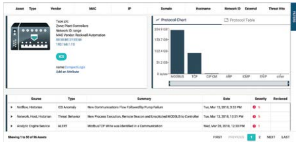
Figure 3: PLC Asset Details
